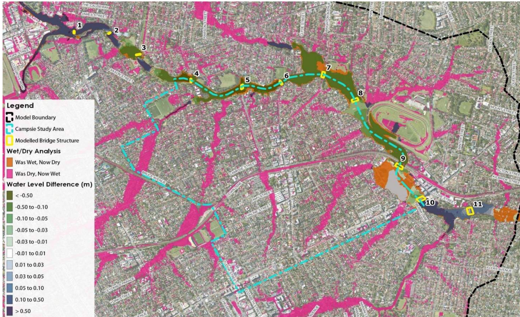
Figure 3-14 Peak Water Level Result Differences (in metres) – 1% AEP Event - Updated Flood Model Less 2009 Mainstream Study Model
